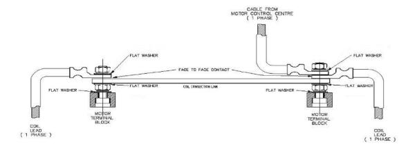
Do not separate your link from your ring terminal with a brass nut or washer, this can create a high resistant joint which can cause motor failure.
