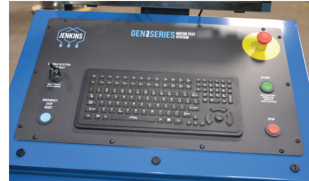
Separate Operator Console allows the user to energize the motor under test and monitor live data at a safe distance.
