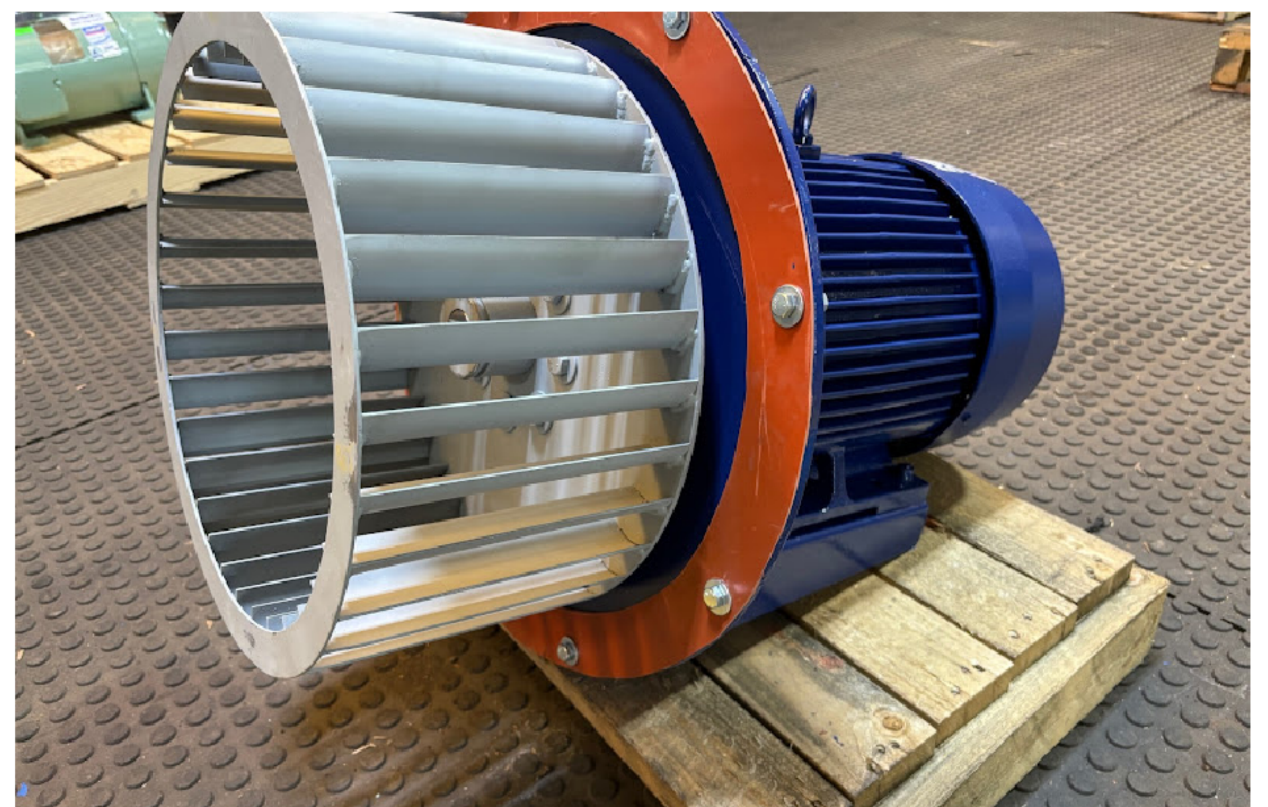
New fan mounted on the motor.
