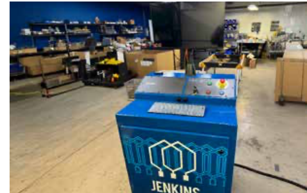
Separate Operator Console allows the user to energize the motor under test and monitor live data at a safe distance.
