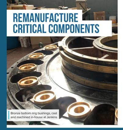
When the part you need is obsolete or hard-to-find, the Jenkins foundry stands at-the-ready. We're able to remanufacture from a sample or print, and cast in aluminum, bronze, brass or copper. The ability to create custom parts is critical for hydroelectric generators, especially when you consider that they serve as some of the oldest power plants in the nation, with the average hydroelectric facility operating for 64 years.
