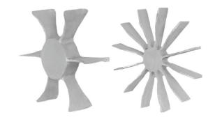
**DIMENSIONS** Overall diameter (D) is most critical in determining air delivery over the motor. Blade width or height (A) is also important, but the number of blades is not significant. Be sure the fan blade you choose clears the bearing housing outside diameter, and the fan cover inside diameter. Tolerances are  $\pm$  1/8" on all dimensions except bore.
