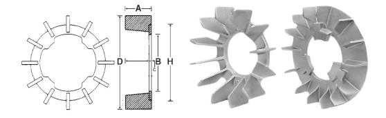
**DIMENSIONS** Overall diameter (D) is most critical in determining air delivery over the motor. Blade width or height (A) is also important, but the number of blades is not significant. Be sure the fan blade you choose clears the bearing housing outside diameter, and the fan cover inside diameter. Tolerances are  $\pm$  1/8" on all dimensions except bore.
